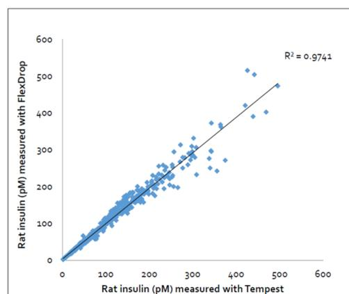
**Figure 2.** Comparison of automated AlphaLISA results measuring insulin concentration in plasma using either Tempest or FlexDrop instruments for the addition of reagents to assay plates.
