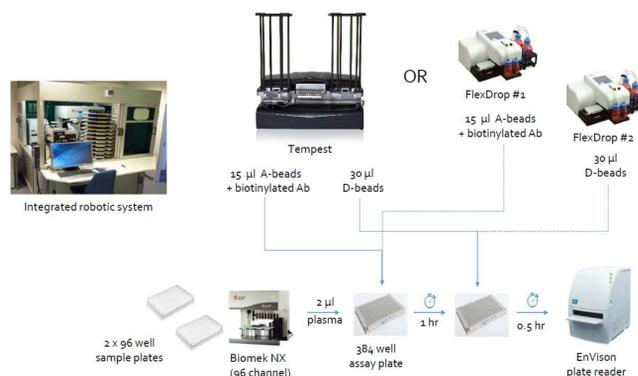
**Figure 1.** Automated AlphaLISA workflow. Plasma samples are transferred in duplicate from 96-well source plates to 384-well assay plate along with calibrators and controls for a total of 144 samples per plate. Assay reagents (Acceptor beads + biotinylated antibody and Donor beads) are added to assay plate using either one Tempest or two FlexDrop dispensers. Photo of the integrated system with robotic arm and incubation/storage racks capable of running 20 assay plates in 6 hours.
